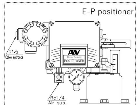
**8 Connection of E-P positioner procedure**
