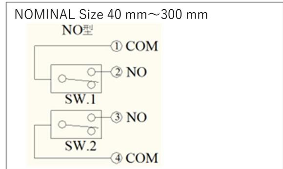
SW.1: Contact closes when valve is closed
