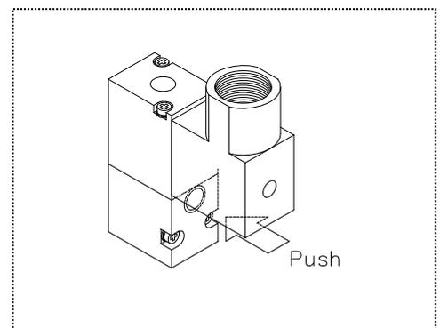
**Adjusting the Opening/Closing Speed <Double acting>**
