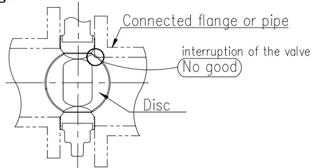
The butterfly valve is designed to be used for piping of various materials. However, especially when a large wall thickness of the connecting part (flange pipe) with the valve is used, it is necessary to chamfer the inner end of the connecting part in order to avoid contact between the valve Disc and the inner surface of the connecting part. There is no problem if the inner diameter of the connecting part is equal to or greater than the following value.
