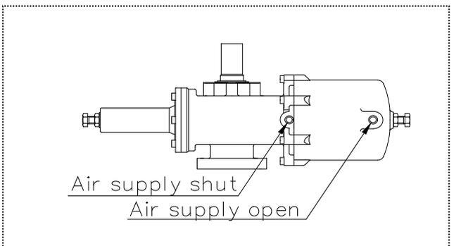
With solenoid valve and regulator with filter
