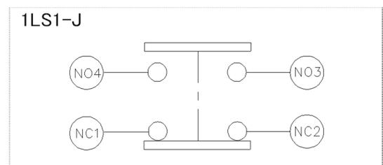
SW.1: Contact closes when valve is closed
