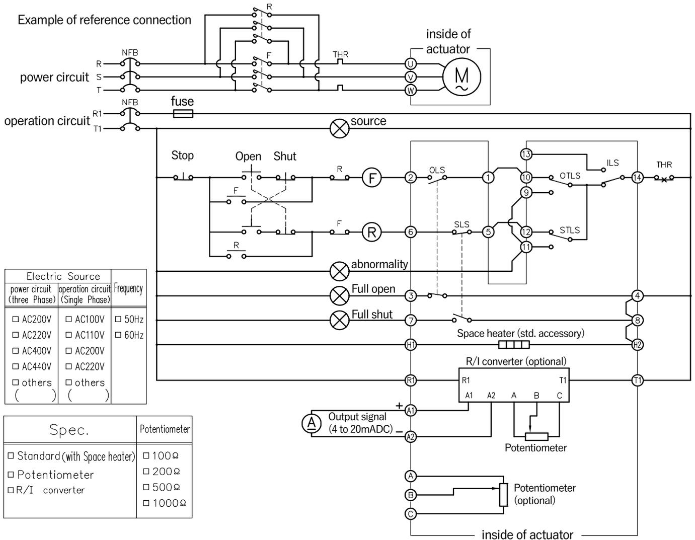
NOTE; The wiring diagram shows the end of the opening operation.
