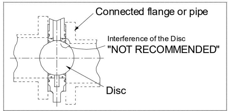
Large bore butterfly valves made of PDCPD are designed to be used for piping of various materials. In particular, when using large wall thicknesses of the connecting part (flange/pipe) with the valve, chamfering of the inner end of the connecting part is required to avoid contacting the valve disc with the inner surface of the connecting part. There is no problem if the inner diameter of the connecting part is equal to or greater than the following value.
