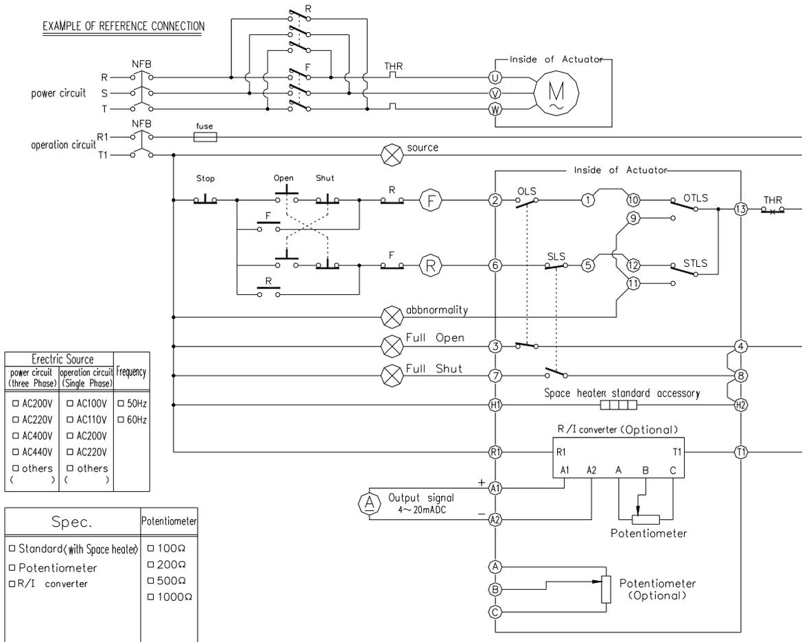
NOTE. This circuit diagram shows the position that the opening action has come to an end.
