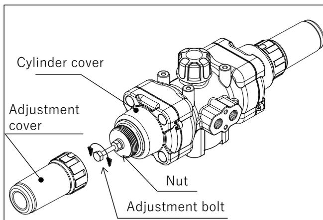
Adjustment angle and number of revolutions of hexagon head bolt (reference) Unit; Rotate
