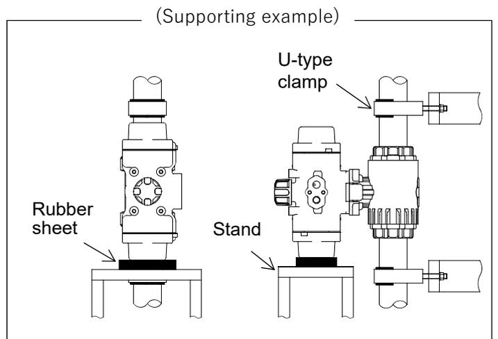
With the conditions that do not require the support of the actuator section
