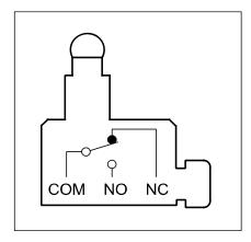
COM-NC is ON when valve right is fully open or left is fully open.
