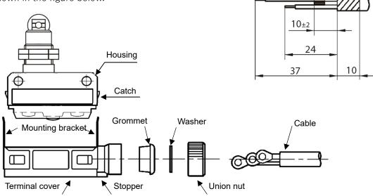
5) Connect the crimp terminal to the terminal by referring to the figure below. When the valve is fully open (or fully closed), COM-NC are ON.
