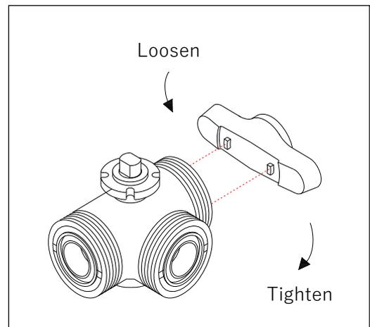
**8. How to disassemble/assemble parts for replacement**
